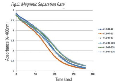
Magnetic separation rate was determined by measuring absorbance over time (Gensys 10S UV-Vis Spectrophotometer, λ = 400nm). Magnefy populations separated rapidly and uniformly.
