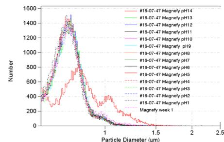
Fig. 6: Sizing under various pH conditions
