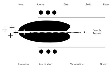
Fig. 4: ICP-MS Concept
