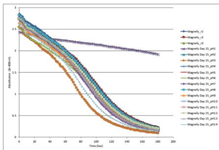
Fig. 7a: Separation under various pH conditions
